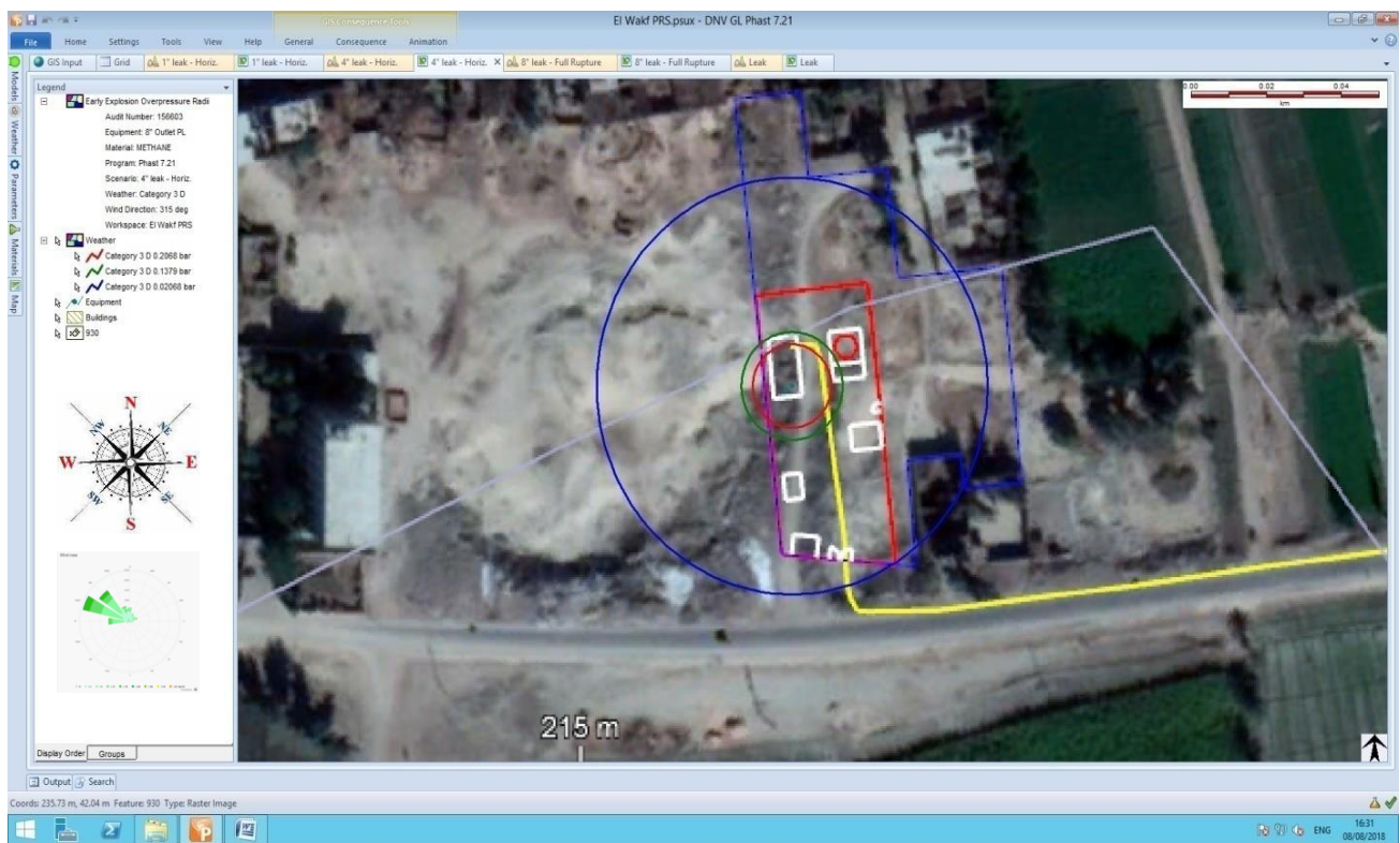
Figure (25) Early Explosion Overpressure Waves (4" hole in 8" Outlet Pipeline)
