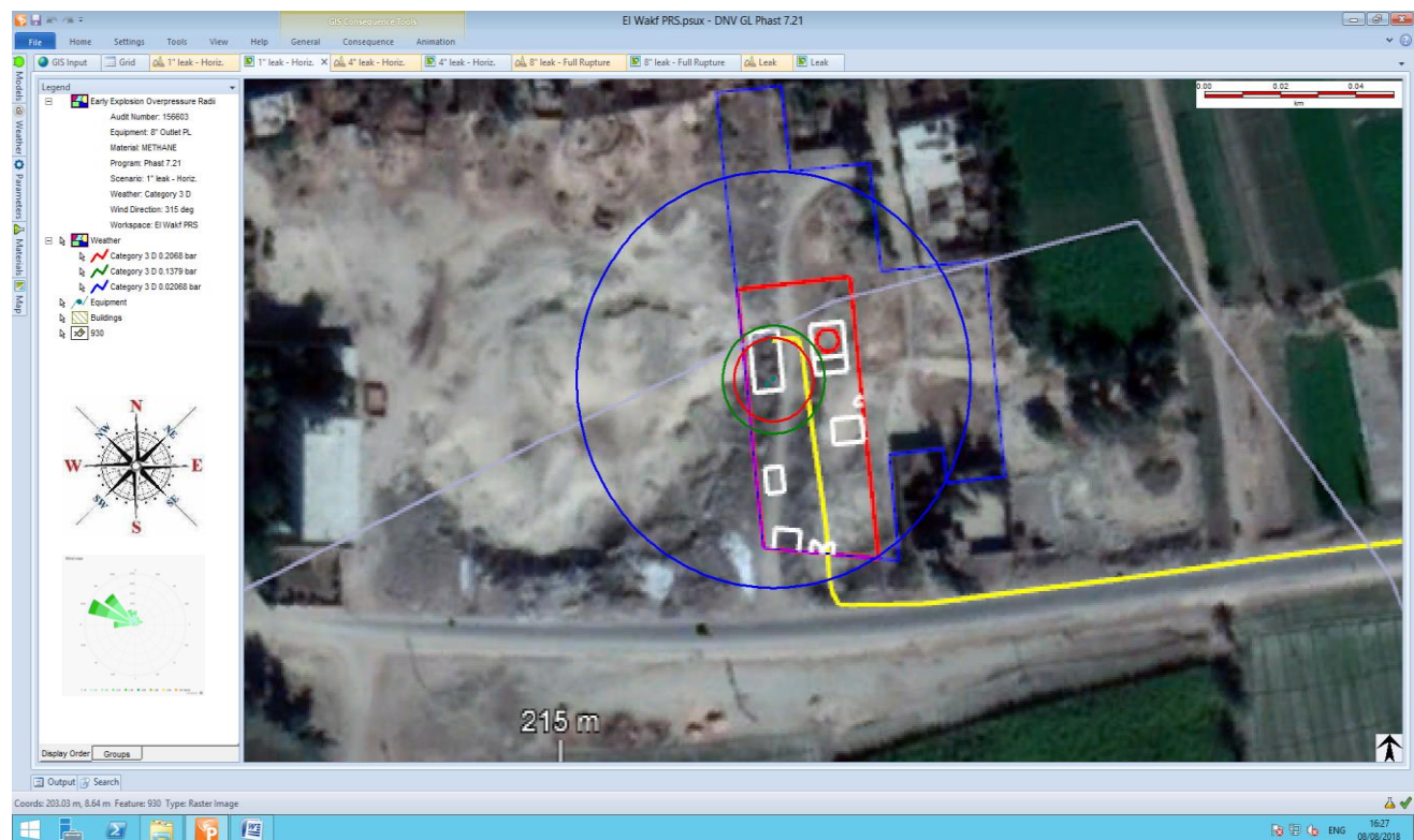
Figure (22) Early Explosion Overpressure Waves (1" hole in 8" Outlet Pipeline)
