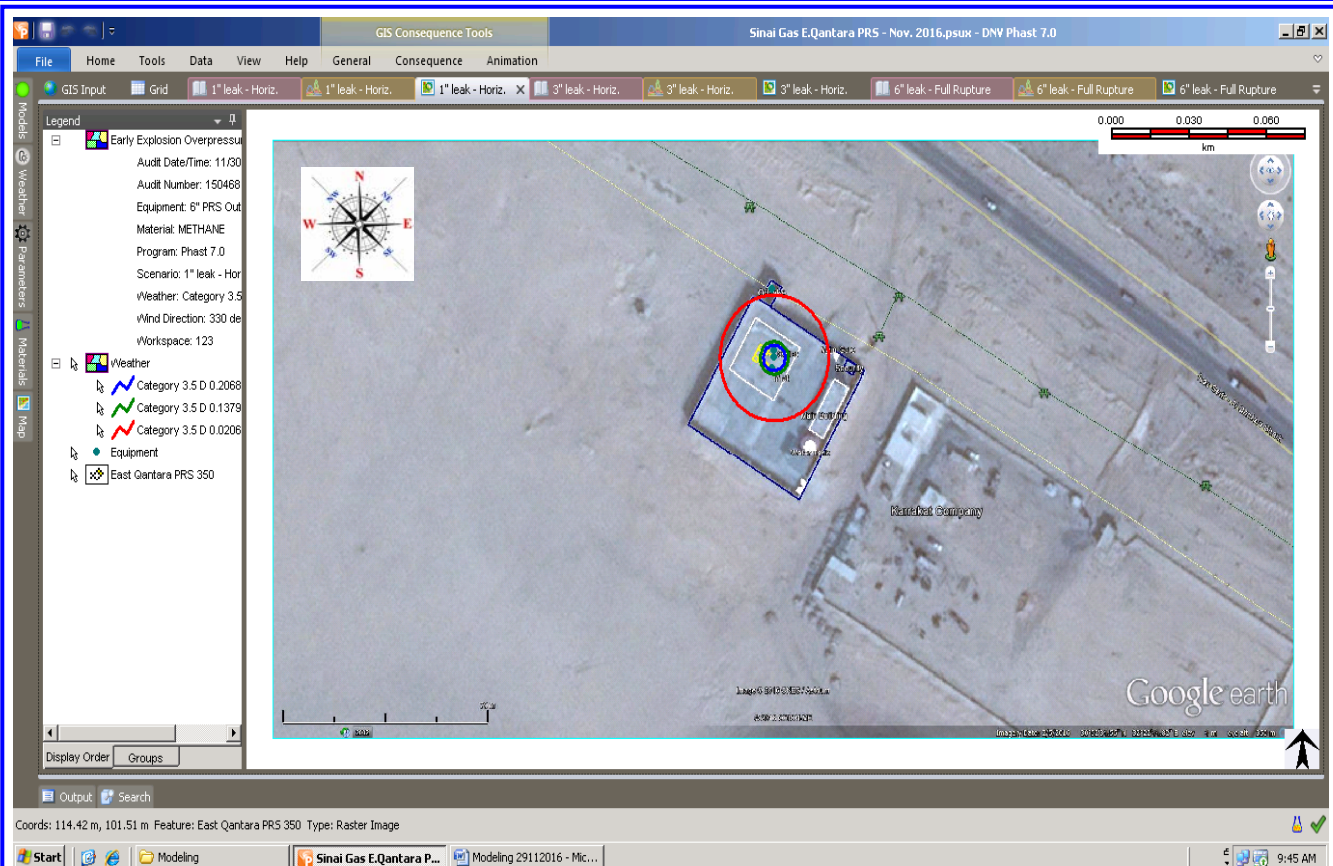
Figure (29) Early Explosion Overpressure Waves (1" hole in 6" Outlet Pipeline)
