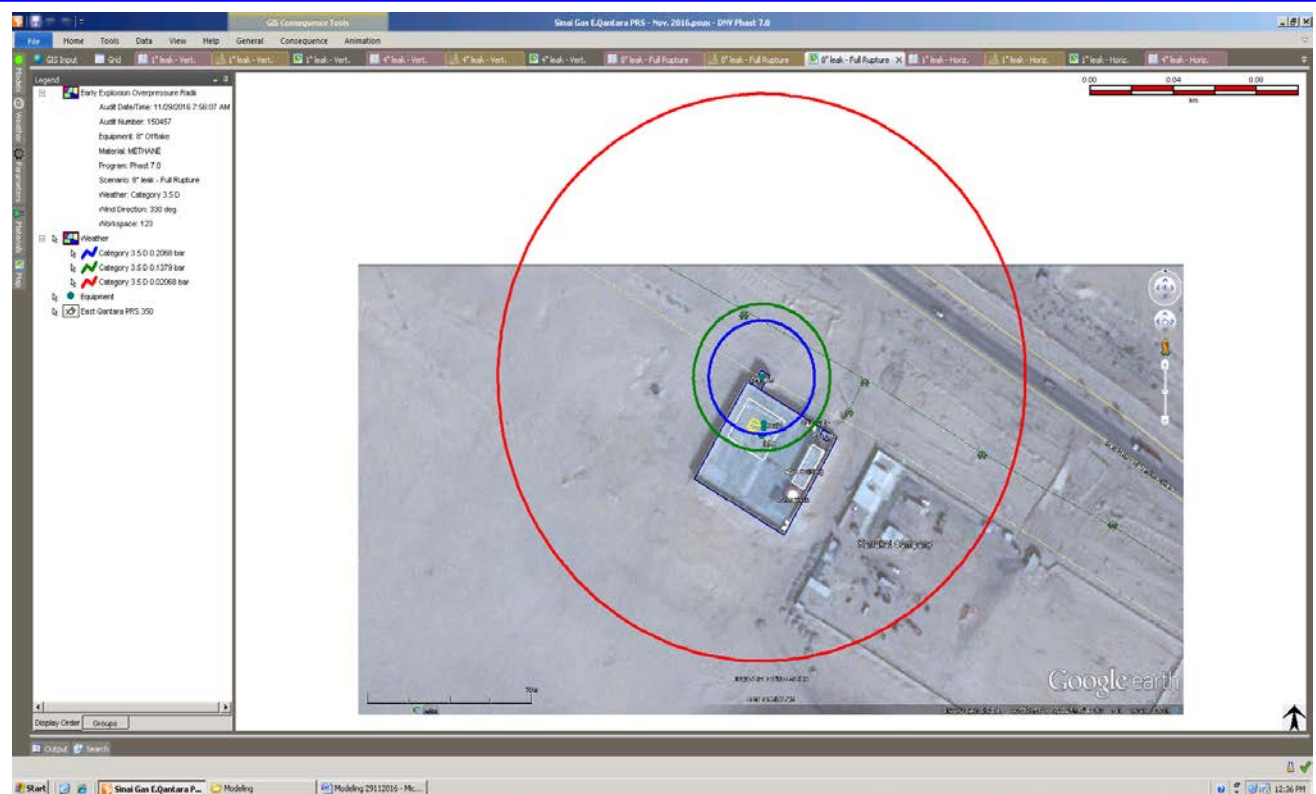
Figure (54) Early Explosion Overpressure Waves (8" off-take Pipeline Full Rupture)
