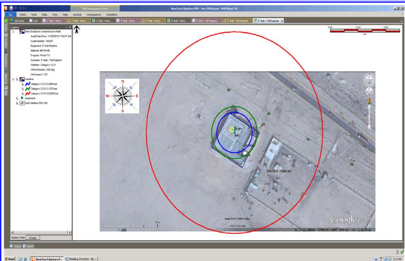
Figure (24) Early Explosion Overpressure Waves (8" Inlet Pipeline Full Rupture)
