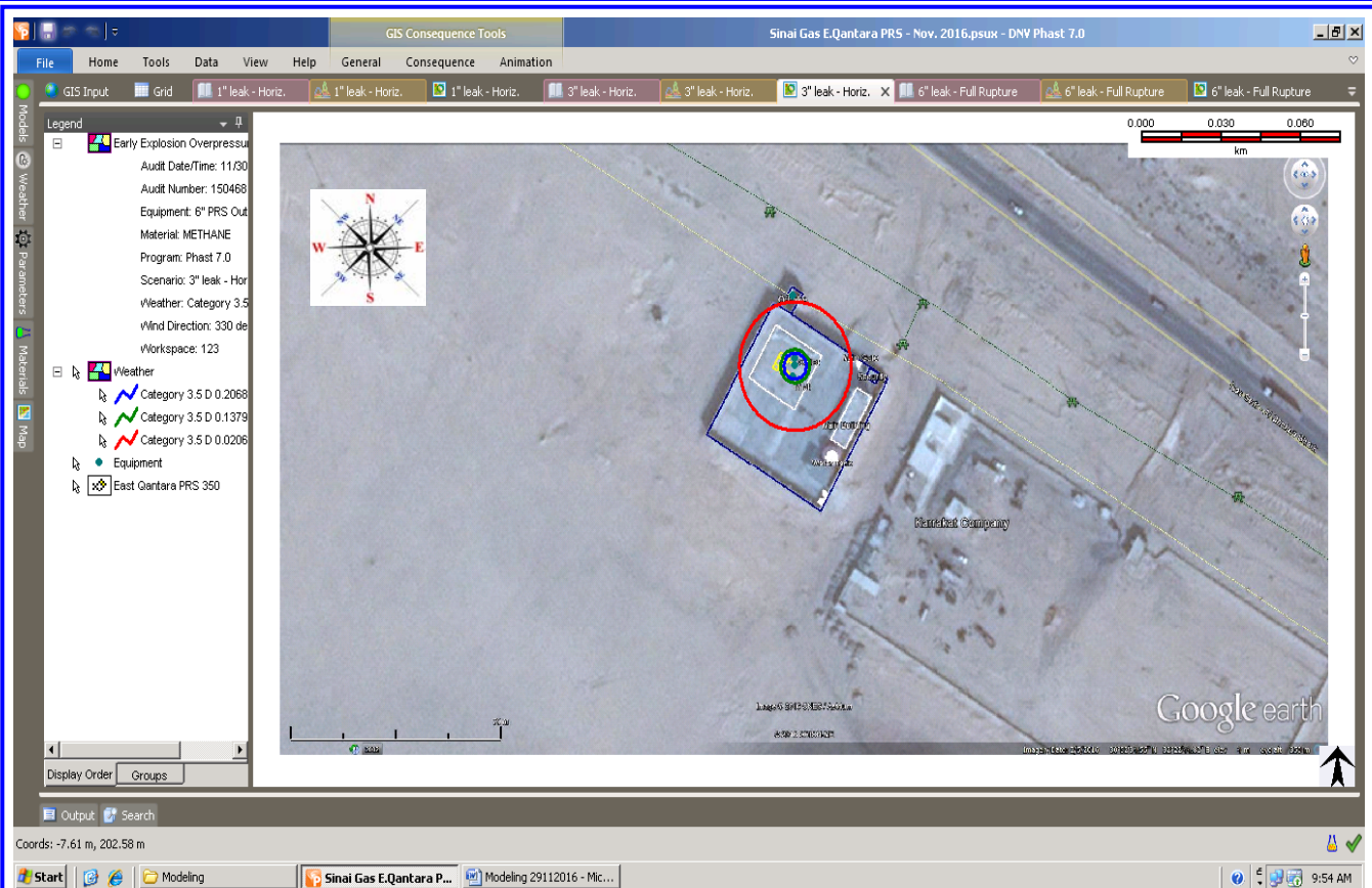
Figure (33) Early Explosion Overpressure Waves (3" hole in 6" Outlet Pipeline)
