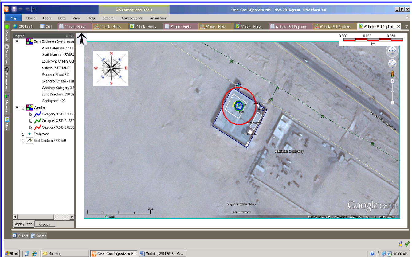
Figure (37) Early Explosion Overpressure Waves (6" Outlet Pipeline Full Rupture)
