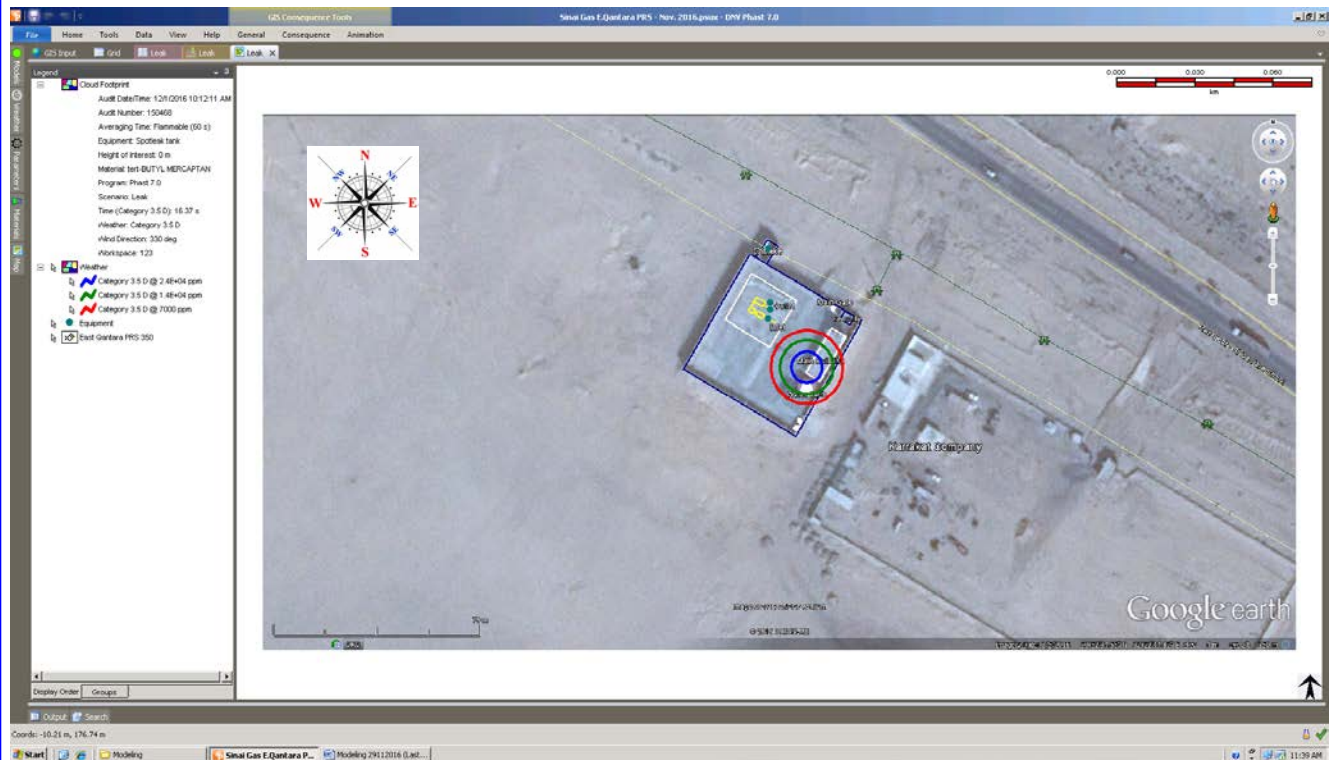
Figure (41) Vapor Cloud (UFL/LFL) Footprint on Site Map (Odorant leak)
