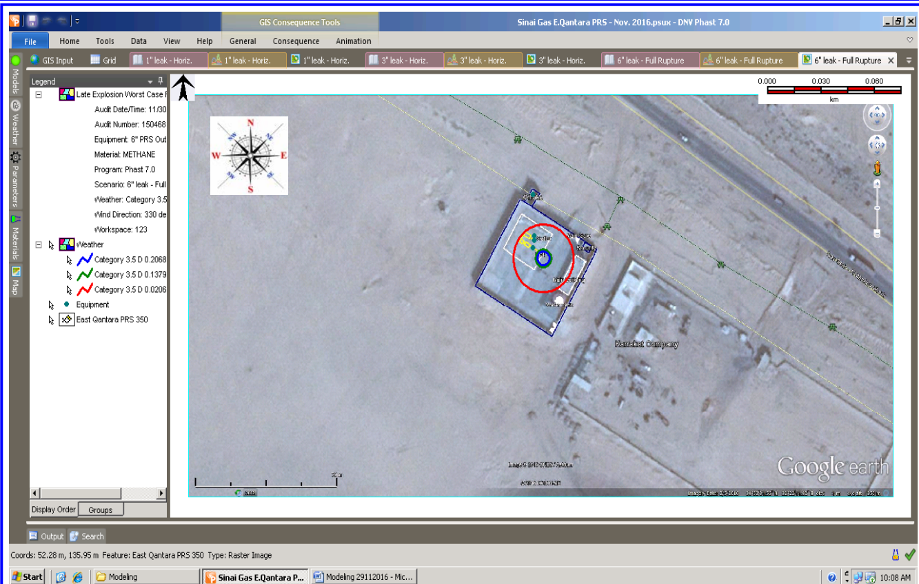
Figure (38) Late Explosion Overpressure Waves (6" Outlet Pipeline Full Rupture)
