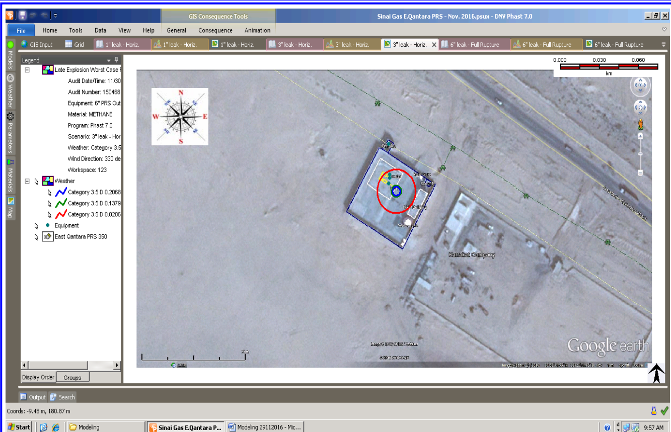
Figure (34) Late Explosion Overpressure Waves (3" hole in 6" Outlet Pipeline)
