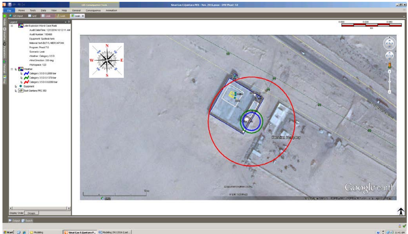
Figure (45) Late Explosion Overpressure Waves on Site (Odorant Leak)
