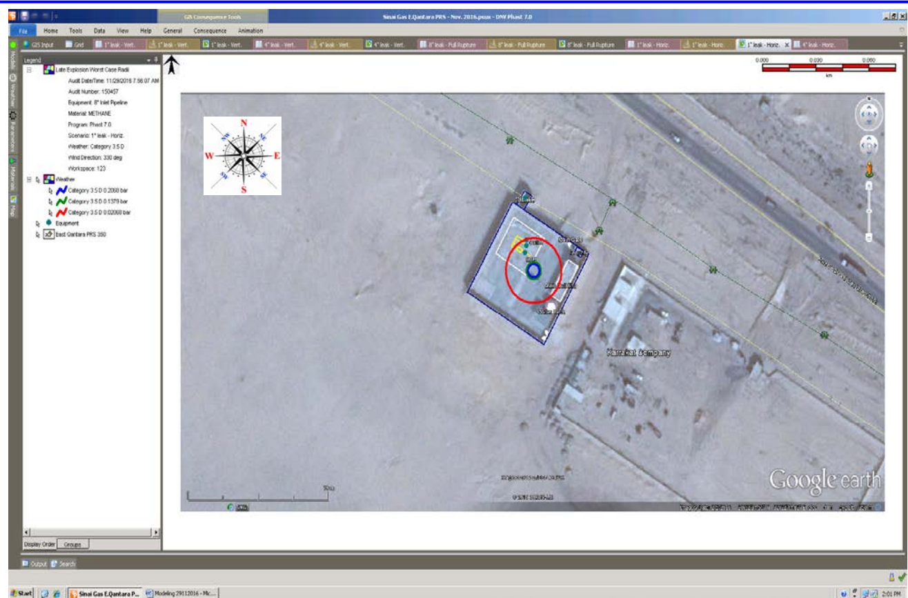
Figure (17) Late Explosion Overpressure Waves (1" hole in 8" Inlet Pipeline)
