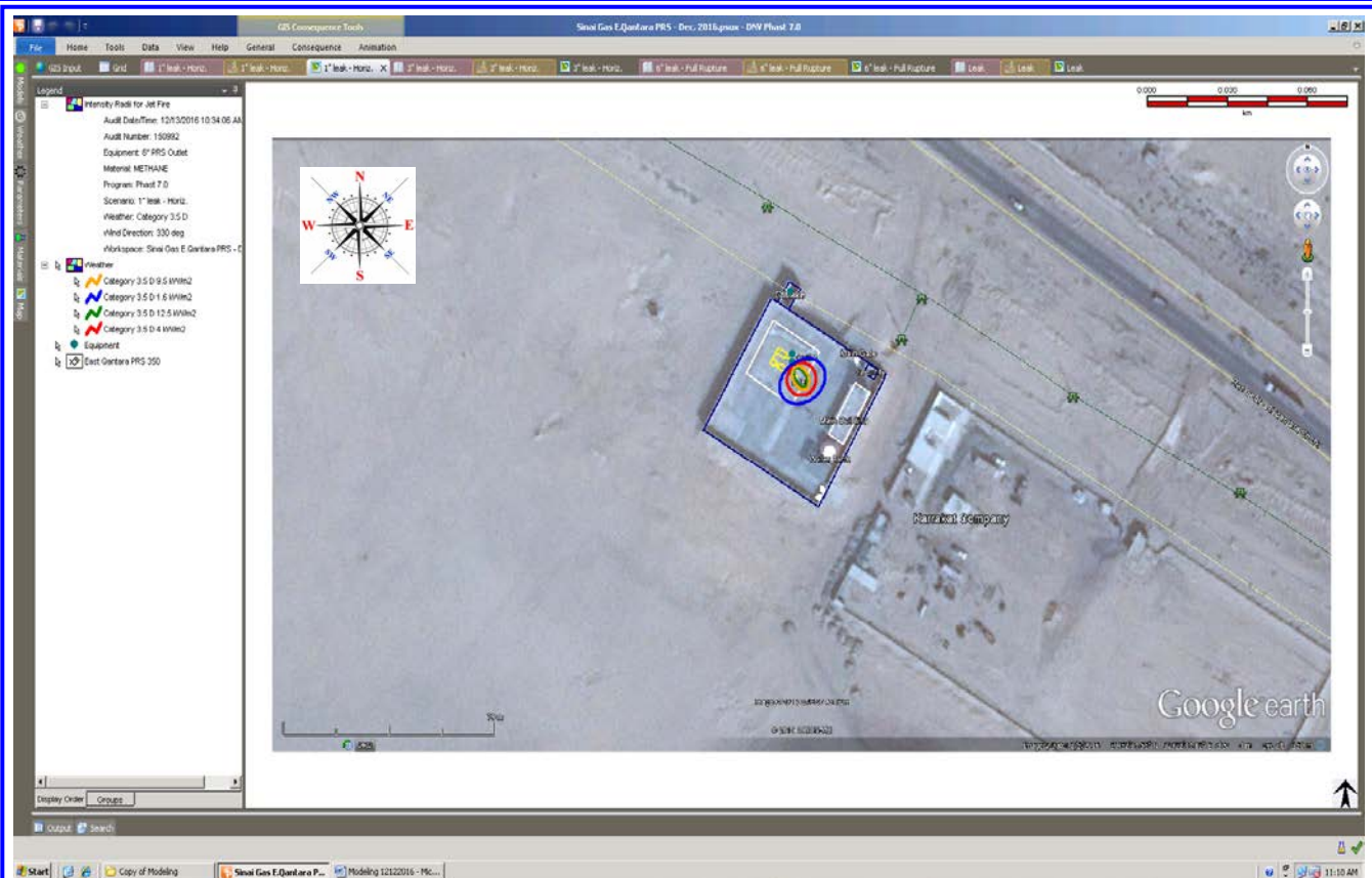
Figure (28) Heat Radiation Contours from Jet Fire (1" hole in 6" Outlet Pipeline)
