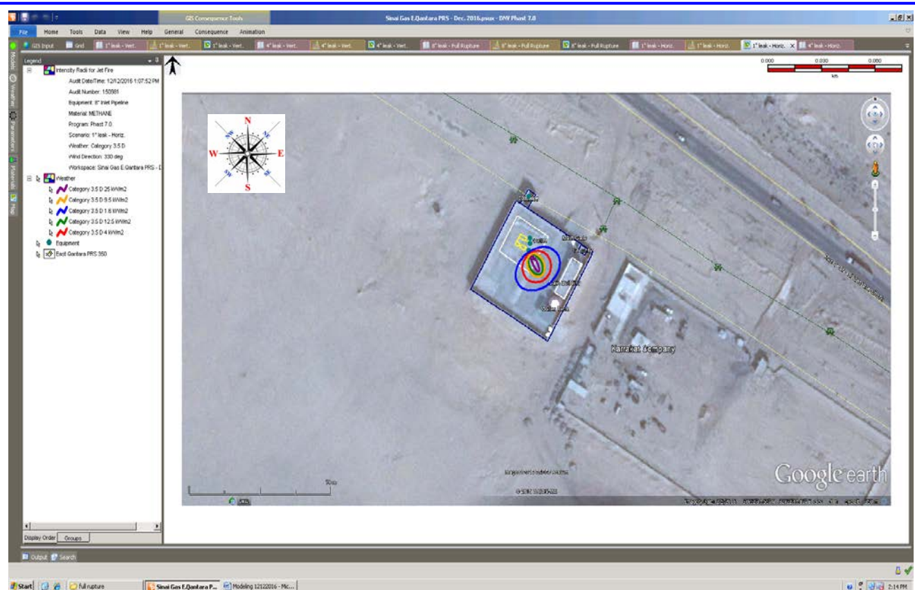
Figure (16) Heat Radiation Contours from Jet Fire (1" hole in 8" Inlet Pipeline)
