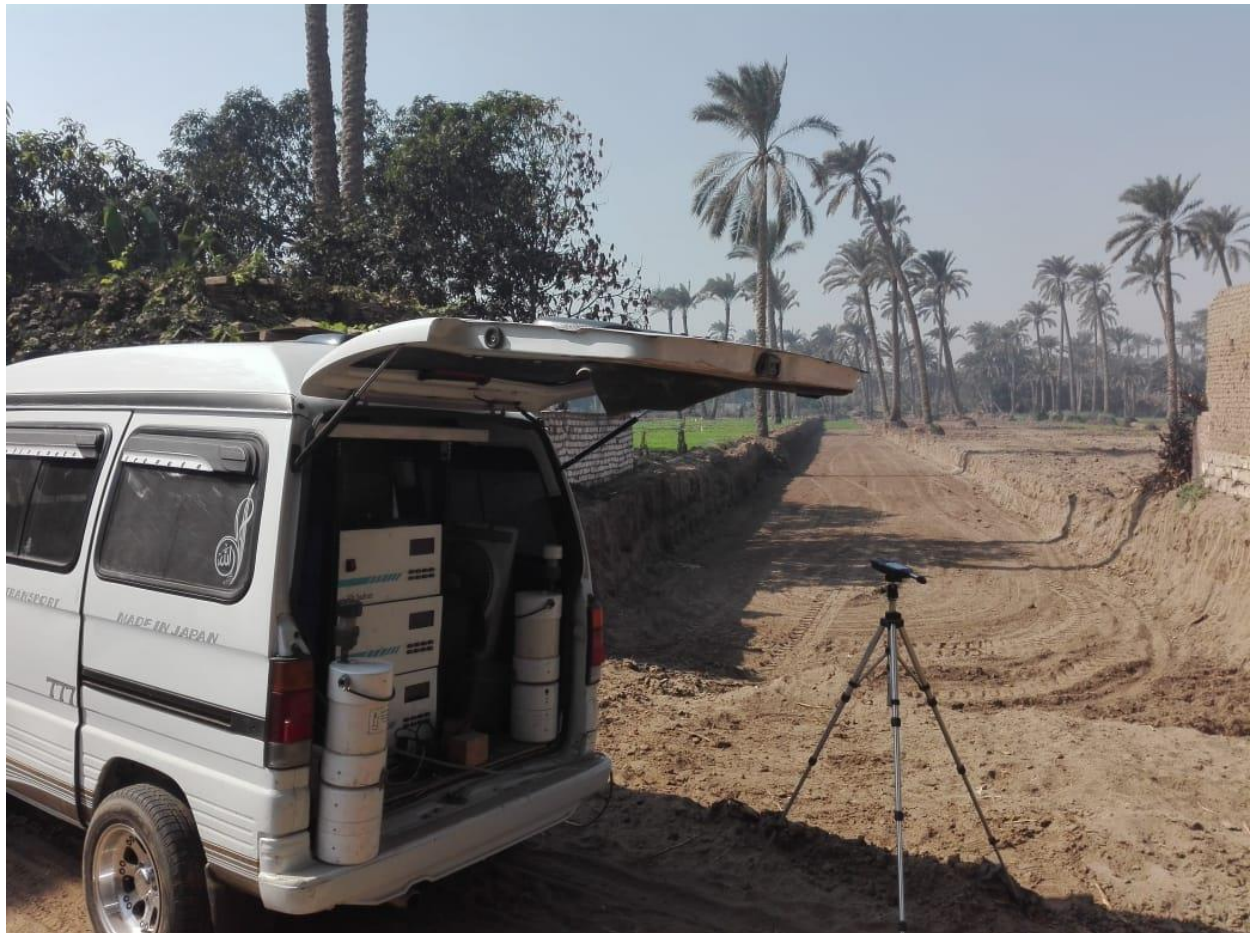
Figure 3-1 ambient air quality monitoring system
